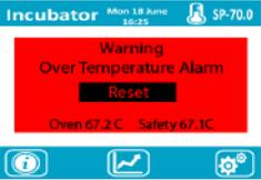
If the unit is set as Auto reset, when the temperature falls below the (Value - Hysteresis) it will automatically reset and continue operations.
