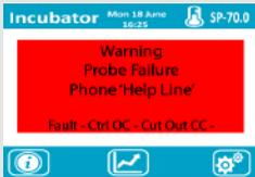
Sensor failure. If the probes are damaged, the control system shall automatically turn the heating elements off.
