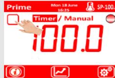
If the chamber is configured with internal lights or extraction systems, these can be manually turned on or off by pressing the play or square icon. See [Output Relay Action - Page 13](#).
