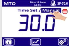
Select to run in either Real Time Clock mode or in Manual mode.
