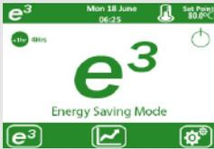
The cabinet will always be in run mode between the hours of 7am and 7pm Monday to Friday. In run mode, it will automatically control to the Set Point. If you don't want to warm the cabinet between these hours, turn off the unit with the on/off master rocker switch. Outside of these hours, the cabinet will be in Energy Saving Mode as shown here and will turn the elements and fans off.
