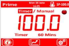
Within 2 deg of setpoint, the chamber will start the count down timer and the remain time is displayed on screen. This time period can be changed between 1 and 5000 minutes in the Timer Configuration section [shown on page 11](#).
