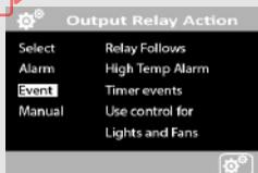
The chamber may be built with an additional siren / beacon or with an oven light that you can control via the touch screen.
