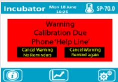
If you requested a calibration certificate with your chamber, the control system shall give you notification when the calibration is about to expire one month before. If you require a new calibration, please contact your supplier.
