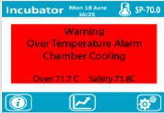
The control system is designed to indicate any faults should they occur.
