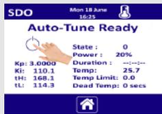
In PID mode, you can manually enter the P, I, and tL and tH value to optimise the control. For fan units, the P is defaulted to 3.000 and for fanless units the P value is defaulted to 1.500. The Integral and tL and tH values are best calculated using the Autotune. Please note the algorithm used in the control system uses Fuzzy Logic. This means these values are constantly updated to provide optimum control.
