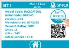
To view chamber information such as serial codes, power ratings, 2nd safety temperature value, press the
