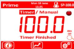
At the end of the countdown, the timer will turn the heat off. Depending on preference, you may choose to turn on a siren/beacon at this stage ([selected in Output Relay Section - Page 13](#)).
