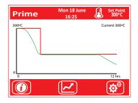
The control system comprises of a bespoke touch screen user interface that offers both accurate temperature control and an integral overheat system by using 2 individual PT100 sensors. Advanced features can be turned on and off to suit bespoke heating applications and tailored to customer preference. Oven trending is displayed for up to 48 hours and optional upgrades are available for alarm outputs.
