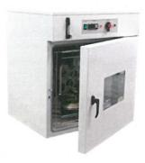
The Rolling Thin-Film Oven (RTFO) procedure provides simulated short term aged asphalt binder for physical property testing. Asphalt binder is exposed to elevated temperatures to simulate manufacturing and placement aging.
