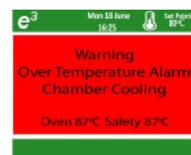
The cabinet will indicate if there is a fault with a diagnostic message. A safety alarm temperature system is designed into the cabinet which will remove power to the elements if the cabinet goes 10 °C above the Set Point. Any alarm messages will appear on the screen. The cabinet will return to normal operation once the cabinet cools below the current Set Point.
