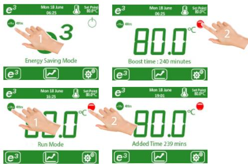
The cabinet will always be in run mode between the hours of 7am and 7pm Monday to Friday. If you don't want to warm the cabinet between these hours, either turn off the unit with the on/off master switch or configure the set point to '0'
