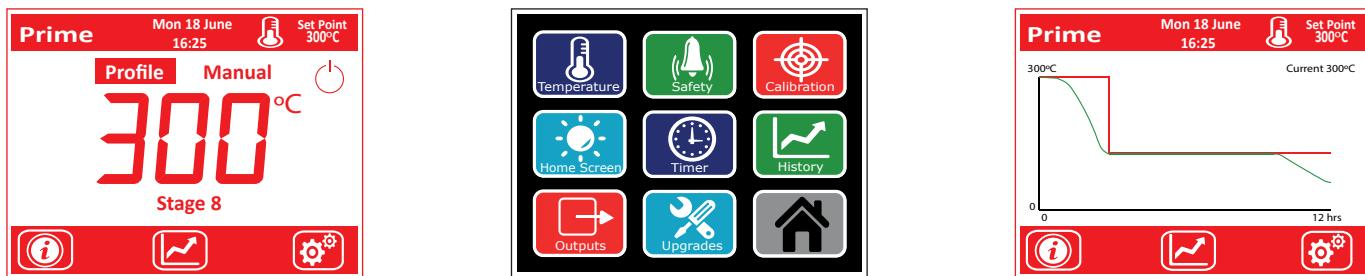
The control system comprises of a bespoke touch screen user interface that offers both accurate temperature control and an integral overheat system by using 2 individual PT100 sensors. Advanced features can be turned on and off to suit bespoke heating applications and tailored to customer preference. Oven trending is displayed for up to 48 hours and optional upgrades are available for alarm outputs.
