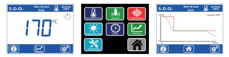
The control system comprises of a bespoke touch screen user interface, that offers both accurate temperature control and an integral overheat system by using two individual PT100 sensors. Advanced features can be turned on and off to suit bespoke heating applications and tailored to customer preference. Oven trending is displayed for up to 48 hours and optional upgrades are available for alarm outputs.
