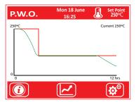
The control system comprises of a bespoke touch screen user interface that offers both accurate temperature control and an integral overheat system by using 2 individual PT100 sensors. Advanced features can be turned on and off to suit bespoke heating applications and tailored to customer preference. Oven trending is displayed for up to 48 hours and optional upgrades are available for alarm outputs.
