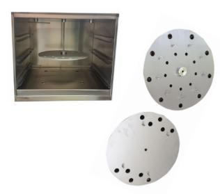
This dual purpose oven is designed to perform the Loss On Heat and Thin Film Test for bitumen and asphaltic materials and complies to the requirements of BS2000 ASTMD6, D1754 & AASHTO T47, T179.
